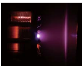
Operation of radio frequency plasma cathode
