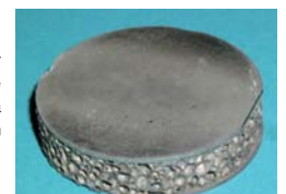
Aluminum foam sandwich manufactured through superplastic diffusion bonding
